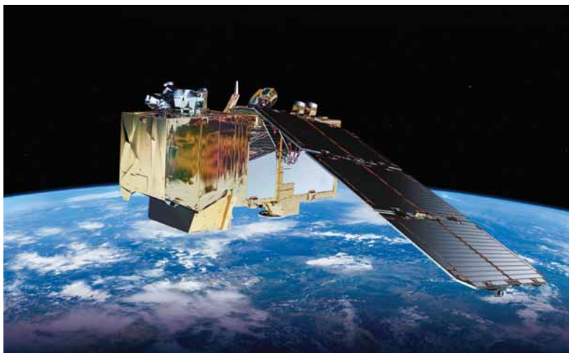
Artist's impression of Sentinel-2A. Sentinel-2A provides well calibrated, high radiometric resolution multispectral measurements in 13 different wavebands, ranging from visible to shortwave infrared, at spatial resolutions from 10 to 60 m, depending on waveband. Source: ESA-Pierre Carril.
