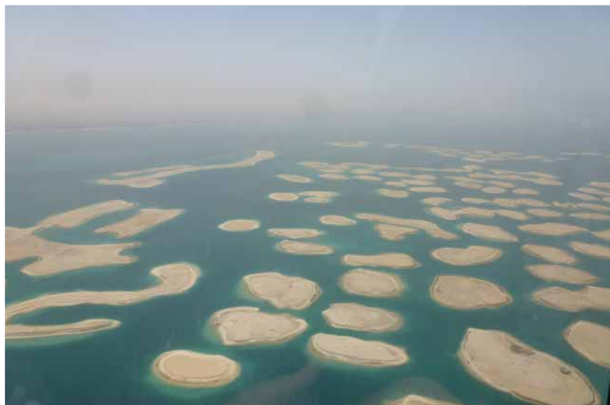
✦ 'The World' group of islands, Dubai, UAE. Taken in April 2015, the image shows the newly constructed archipelago of undeveloped islands. Sand was dredged from the shallow coastal sea bed and pumped to create the islands, protected by long rock breakwaters (discontinuous to prevent stagnation) as seen in the inset below. Source: By Zlatko - Own work, CC BY-SA 3.0, https://en.wikipedia.org/w/index.php?curid=46566985 .
