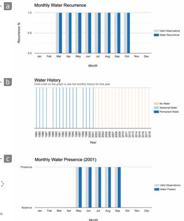
Figure 2-7. Temporal profiles for an area of the Aral Sea; a. Monthly Water Recurrence b. Full Water History (1984-2018) c. Monthly Water Presence (i.e. 1 year's record) The 35-year stack of monthly water classifications at the pixel level form the basis of the water history. The water history is used to create 6 maps, each of which depicts a different facet of surface water distribution over time (see above).
