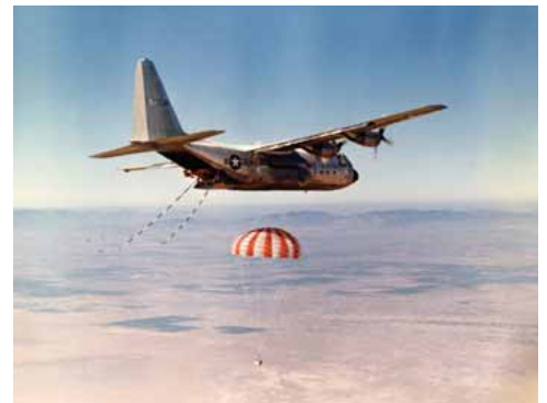
⋯ Catching a satellite. An Air Force JC-130B catching a satellite with grapple gear and winch at Edwards AFB, California, 1969. Source: United States Air Force (Public domain)
