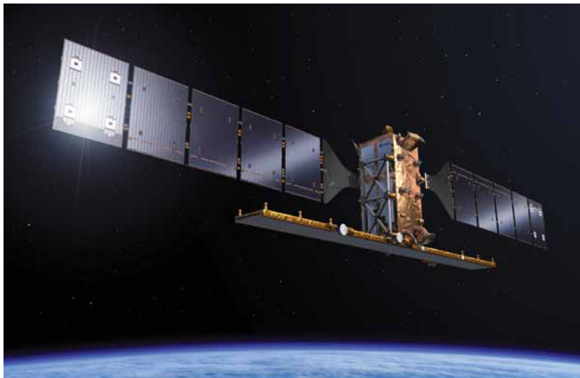
Artist's impression of Sentinel-1B. Radar satellites, such as Sentinel-1B, provide all-weather, day and night imaging capabilities. Source: ESA-Pierre Carril.
