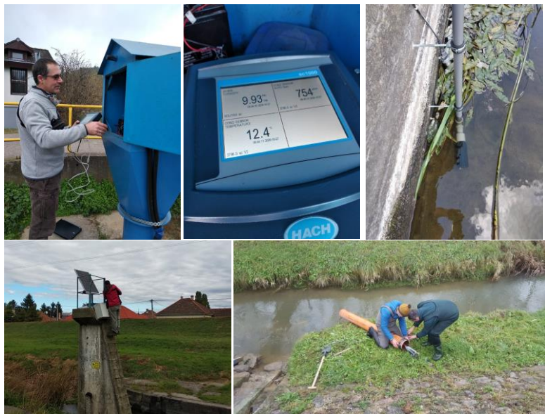
Fig. 1: Setup of online monitoring stations (Photo assembly the Hungarian team)
