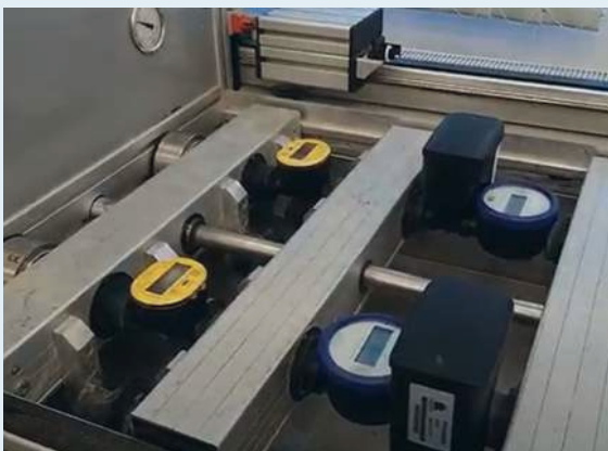
Prototypes of the innovative smart metering developed within the framework of the project
