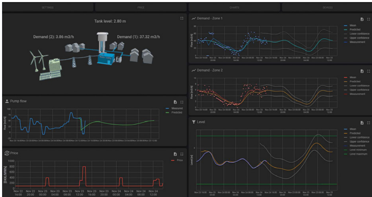
Figure 2.2-6 – Cloud-based solution visualised on an open-source IoT platform (Thingsboard, Inc., 2016). The dashboard shows demand and level predictions along with the flow scheduling of the pumps
