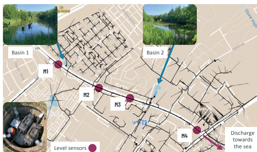
Figure 2.2-1 – Stormwater network in Ishøj, where red dots denote the placement of water level sensors (M1-3.)
