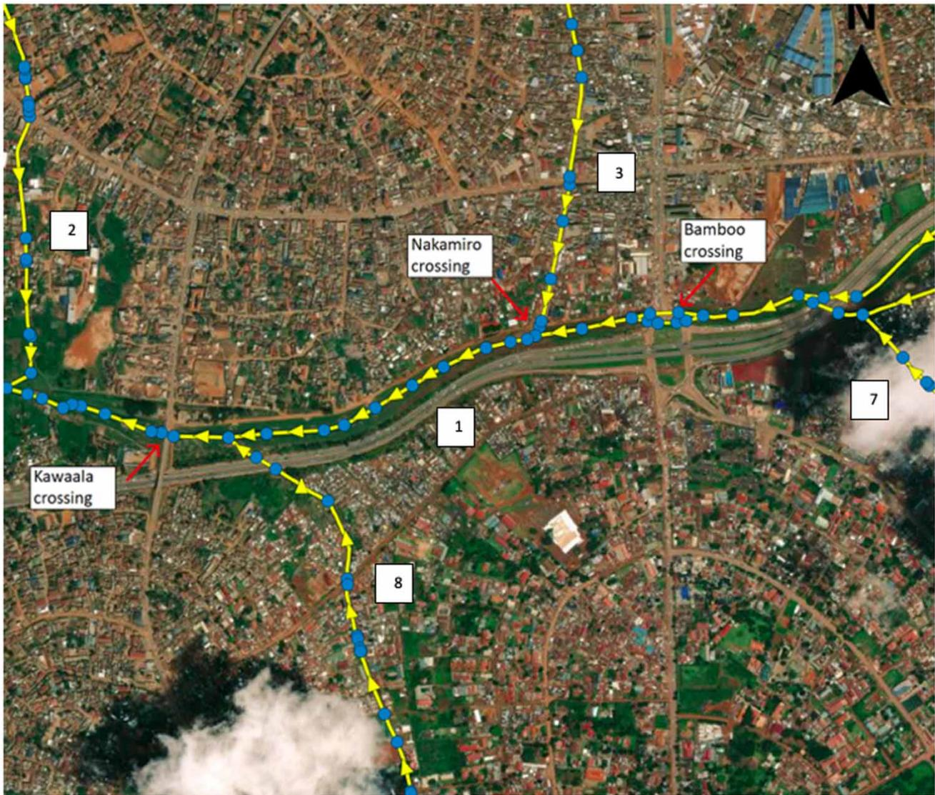
**Figure 10** | Culvert crossings with increased sediment and solid waste blockage, used for Scenarios 2 and 3. The numbers next to the channels are the same as in the overview, shown in Figure 6. Kawaala and Bombo Road crossings are located on the primary channel (1), and Nakamiro crossing is located on a secondary channel (3).
