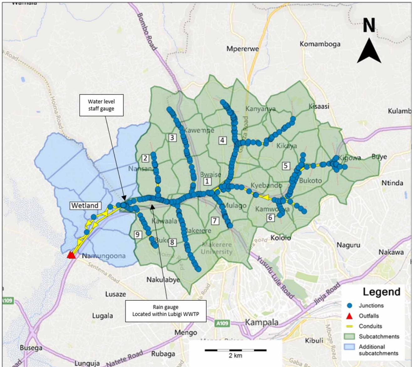
**Figure 6** | Overview of the modelling setup in PCSWMM showing the primary open channel (1) and eight secondary channels (2–9). The catchment area (green) is delineated into 35 sub-catchments and extended with eight more additional sub-catchments (blue) to account for water downstream that could affect the upstream catchment area.
