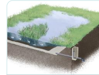
Free water surface treatment wetland
