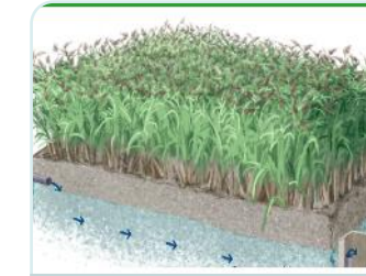
Reactive media in treatment wetland
